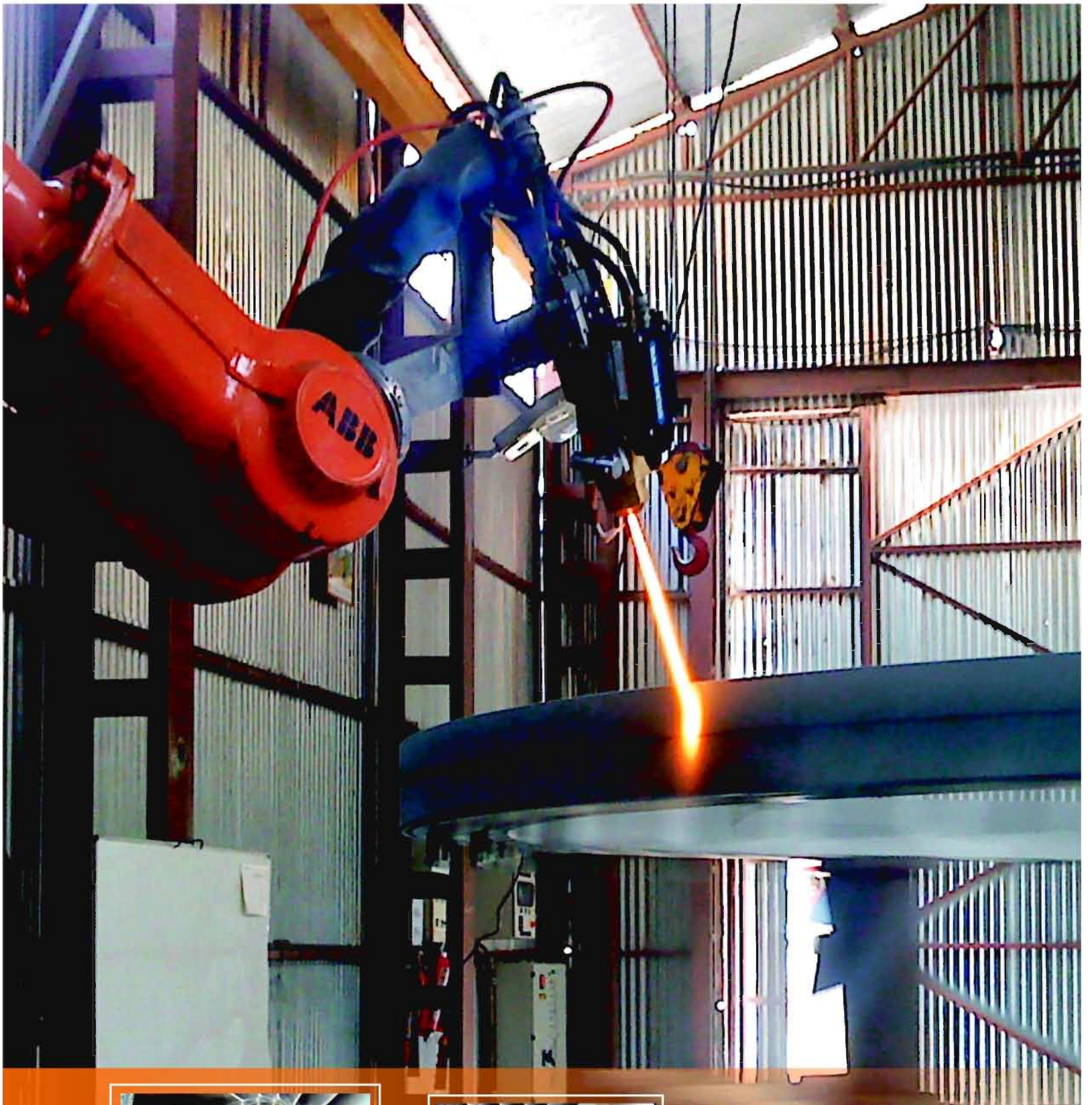
The HVOF coating workshop established at NJHPS. The damaged and repaired parts (inset)
