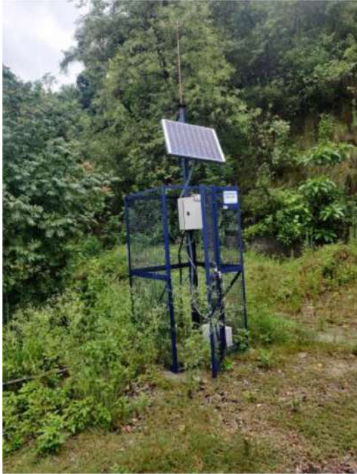
Photo 1- Early flood monitoring devices at Neugal Khad
