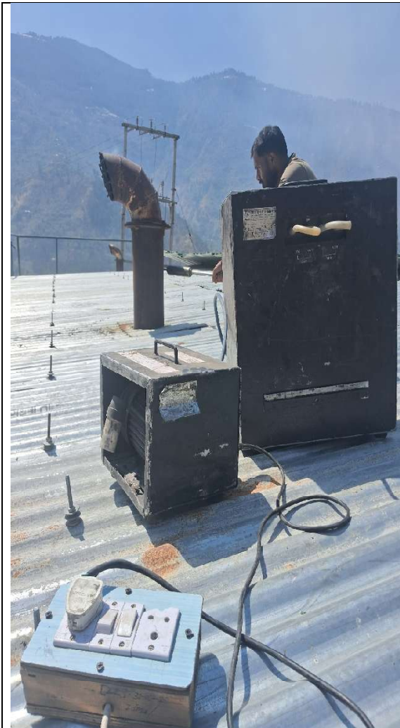
On-site technicians conducting stack/source emission monitoring on the facility's exhaust system to ensure compliance with environmental air pollution standards.
