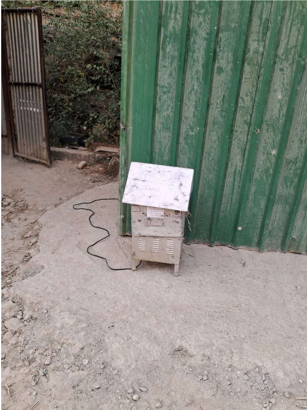
Third-party environmental monitoring equipment positioned at a vulnerable site boundary interface. This setup continuously monitors ambient air parameters ( \{PM\}_{10} and \{PM\}_{2.5} ) to scientifically validate the efficacy of ongoing on-site dust suppression measures (such as systematic water sprinkling) in arresting fugitive dust, as referenced in Test Report No. 110326N-E-001.
